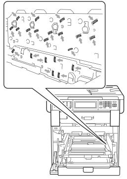
Hold the green handles of the drum unit when you carry it. DO NOT hold the sides of the drum unit. Wipe the four scanner windows (1) with a dry, lint-free cloth.
